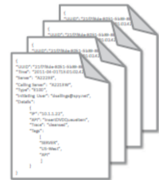
Document data model Collection of complex documents with arbitrary, nested data formats and varying "record" format.
